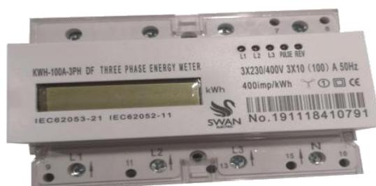
The meter is used in three phase four wire /three phase three wire /two phase three wire power grid. The meter is designed to measure AC active energy. All of its functions comply with the relative technical requirement for class 1 three phase watt hour meter in IEC62053-21. It is a long life meter with the advantage of high stability , high over load capability , low power loss and small volume.
