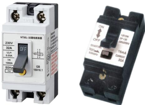
Earth leakage circuit breaker ADNT50LE is suitable for the circuit of AC 50/60Hz, rated voltage 230V, and rated current up to 32A. It is used for protection of the overload and short of all kinds of modern family applicable apparatus. It can also be used for unfrequently operation and control. And this product conforms to IEC61008. 1 standard.
