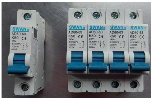
The product is mainly used in AC 50Hz/60Hz single pole 240V or two, three, four-pole 415v circuit for overload and short-circuit protection as well as for infrequent on-and-off switching electric equipment and lighting circuit under normal condition. It is characterized with novel structure, light weight, reliable performance, high breaking capacity. It is in conformity with IEC60947-2 standard.
