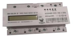
The meter is used in three phase four wire /three phase three wire /two phase three wire power grid. The meter is designed to measure AC active energy. All of its functions comply with the relative technical requirement for class 1 three phase watt hour meter in IEC62053-21.
